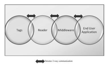
Fig. 1. RFID Infrastructure Components
