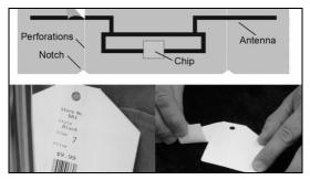
Fig. 6. Clipped Tags (Source:[39]:http://www.gizmag.com/go/5865/)
